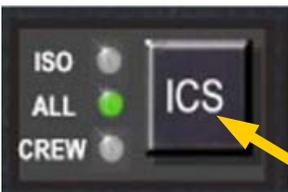
This button cycles through the intercom modes, from top to bottom, ISO, ALL and Crew. An LED shows which mode is currently active.
