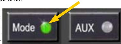
The entertainment inputs automatically mute when there is radio traffic or intercom conversation. In many cases, the muting is not desired, so mute inhibit, or “Karaoke Mode” is available. This is accomplished for the crew by pressing the “Mode” pushbutton. The unit can be wired so that AUX will put the music 2 music into Karaoke mode for the passengers. An external switch located by the passengers can also be installed in lieu of the AUX button function.
